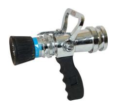
Select Flow nozzles allow the operator to control the flow of the nozzle, depending upon operational requirement, and also give different discharge patterns, from hollow jet (for long range firefighting) to wide fog (for radiant heat protection). Can be used for water or foam operation, and ball valve provided can be used for complete shut off
